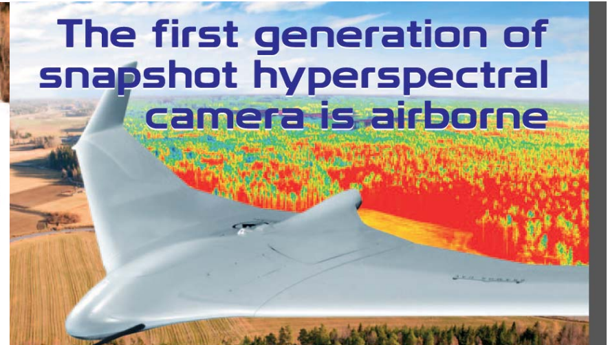
Rikola Hyperspectral imager for light weight UAVs. Ref. www.rikola.fi
