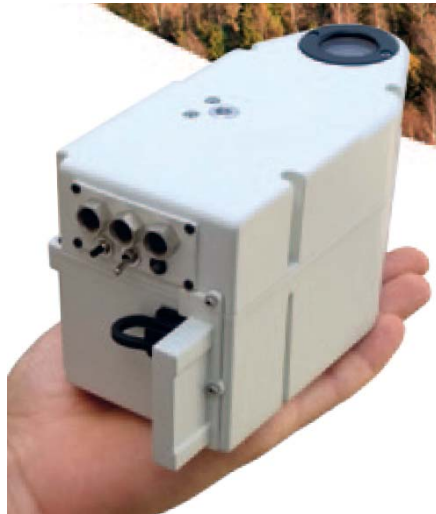
Rikola Hyperspectral imager for light weight UAVs. Ref. www.rikola.fi
