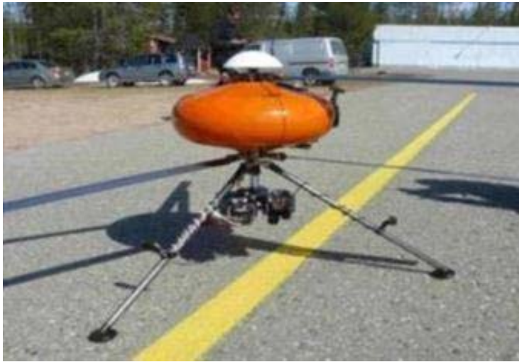
Infotron IT-180 UAV helicopter with max payload capacity of 5 kg
